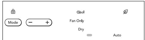
Pressing and holding the Mode button for 3 seconds will activate or deactivate the Lock function. The control panel will be locked and settings cannot be changed.
