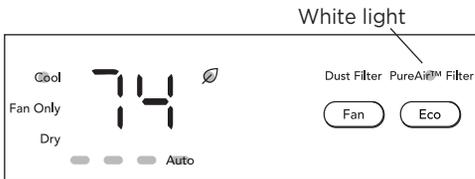
Note: The PureAir™ Filter indicator will glow white, if a PureAir™ filter is installed.
