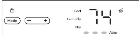
In this mode, the air conditioner will work like a dehumidifier, but will still cool the room. The temperature can be adjusted between 60 °F (16 °C) and 90 °F (32 °C) and the fan speed will be held at Auto speed. Each time Dry mode is selected Eco feature will be activated as default. Press Eco button to deactivate.
