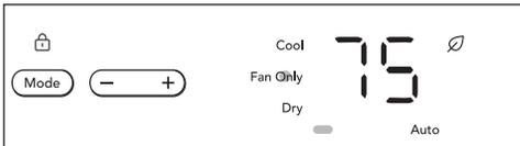
Use this function when cooling is not desired, such as for room air circulation or to exhaust stale air. You can choose any fan speed you prefer. (Except "Auto Fan"). When operating in this mode, the display will show the actual room temperature and the set temperature cannot be changed.
