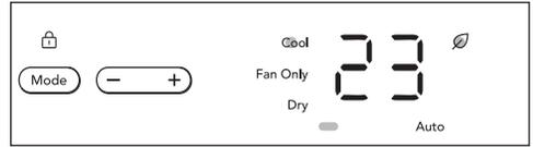
Note: The control is capable of displaying temperature in degrees Fahrenheit or degrees Celsius.
