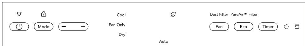
After 60 seconds of control inactivity the display and indicator lights will turn off. Press any button on the control panel or remote control and the display will resume. Please note that if the unit is in Eco feature and the set temperature has been reached the unit may appear off. However, the unit is on and will continue to sample the air every 10 minutes. To confirm, press any button on the control panel or remote control to illuminate the display to show unit in Eco feature.
