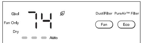
This feature is a reminder to clean the Dust Filter (See Care and Cleaning). The Dust Filter light will illuminate after 250 hours of operation. To reset after cleaning the filter, hold the "Fan" button for 5 seconds.
