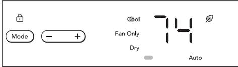
Each time Cool mode is selected, the ECO feature will be activated by default. Press ECO button to deactivate. When ECO feature is deactivated, the fan remains On all of the time with the compressor cycling on and off when the desired room temperature is reached.
