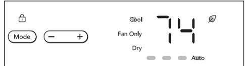
The display will show the set temperature during normal operation, press either up (+) or down (-) buttons to adjust the temperature to desired setting. If the up (+) or down (-) button is pressed continuously, the unit will beep twice when the temperature setting reaches the upper/lower limits 90°F or 60°F.
