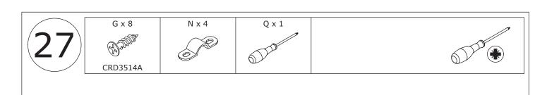
Settle wire using  $\operatorname{clip}(N)$  and fix with  $\operatorname{screw}(G)$  .
