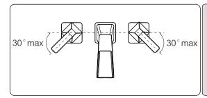
Notice:In order to have the perfect condition of the water flow,please turn both handles to 30 degree angle slowly so that the air inside the tubes can be clean when you use this product at the 1st time.
