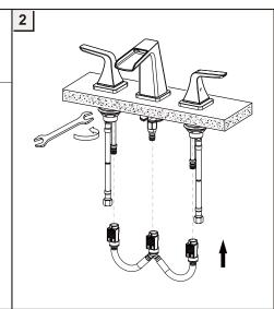
2.Use hand to screw up the locknut, then use install tool for fixing strengthen. And then connect the outlet hose as shown.
