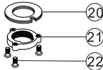
2. Assemble clamp (20) and locknut (21) to faucet shank by hand and tighten the screws (22) with the screwdriver.
