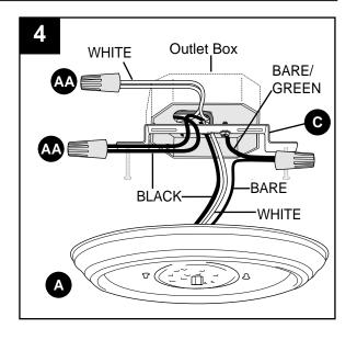
5. Wrap electrical tape (not included) around each individual wire connector (AA) down to the wire.
