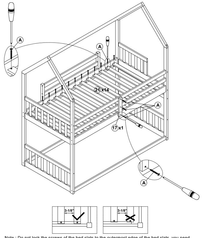
Note: Do not lock the screws of the bed slats to the outermost edge of the bed slats, you need to leave a certain space at the edges, otherwise it will cause the board to break
