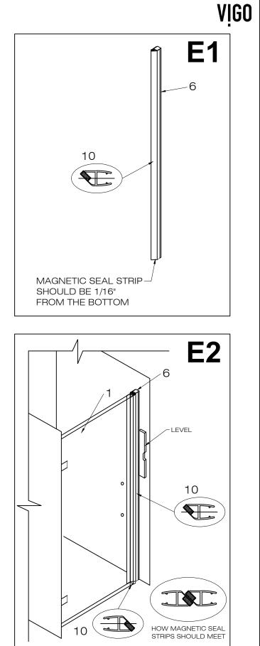
Mark the wall on both sides of the vertical track (#6). The vertical track should be installed with the bottom resting on the floor
