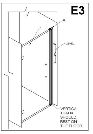
4. Remove the magnetic seal strip (#10) from the vertical track (#6). Hold the vertical track up to the wall where you previously marked and mark the wall through the holes in the vertical track (#6) for installation.
