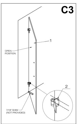
4. Remove the door and drill holes into the wall where marked. Place plastic anchors (#8) inside the holes. <u>Not necessary if installing into studs</u>. Studs are the preferred means of installation, anchors can pull out of the wall causing property damage and bodily harm.
