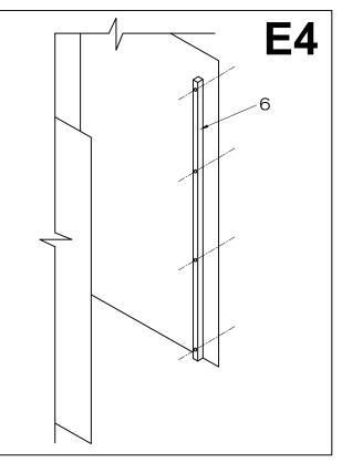
5. Remove the vertical track, pre-drill and sink plastic anchors (#11) into the wall. <u>/Not</u> necessary if installing into studs. Studs are the preferred means of installation, anchors can pull out of the wall causing property damage and bodily harm.
