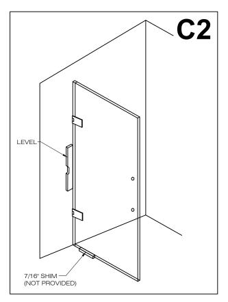
Hold the door in the open position and mark two (2) holes on the wall for the mounting screws for each hinge.
