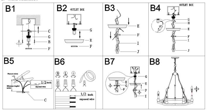
Step B1: .Attach the single bar (E) to outlet box with mounting screws (B). The side of single bar marked "GND" must face out
