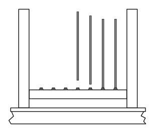
**Step 5:** Place top rail (2x4) over balusters. Install cap rails for a finished look. For rail sections longer than 4 feet, support blocks are recommended. These can be made from leftover rail material. Properly position the support block and toe-nail it to the bottom rail and deck board.
