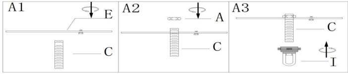
Step A1: Thread the single bar(E) over the nipple (C) a minimum of 6 mm (1/4"). At this point need note that: the side of single bar marked "GND" must face to the down.
