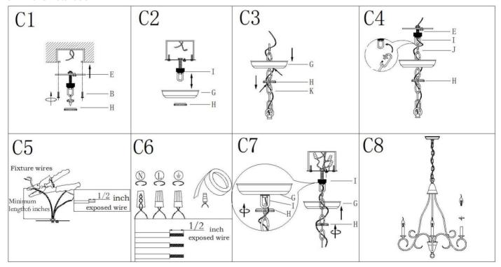
Step C1: .Attach the single bar (E) to outlet box with mounting screws (B). The side of single bar marked "GND" must face out Unscrew the collar ring (H) from the collar loop
