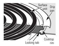
When properly seated, the locking tab should lock onto the cooktop rim through the notch in the drip pan.
