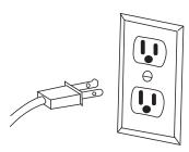
To reduce the risk of electrical shock, this saw has a polarized plug (one blade is wider than the other). This plug will fit in a polarized outlet only one way. If the plug does not fit fully in the outlet, reverse the plug. If it still does not fit, contact a qualified electrician to install the proper outlet. Do not change the plug in any way.
