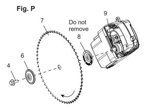
Installing the Blade (Fig. N, O, P)
