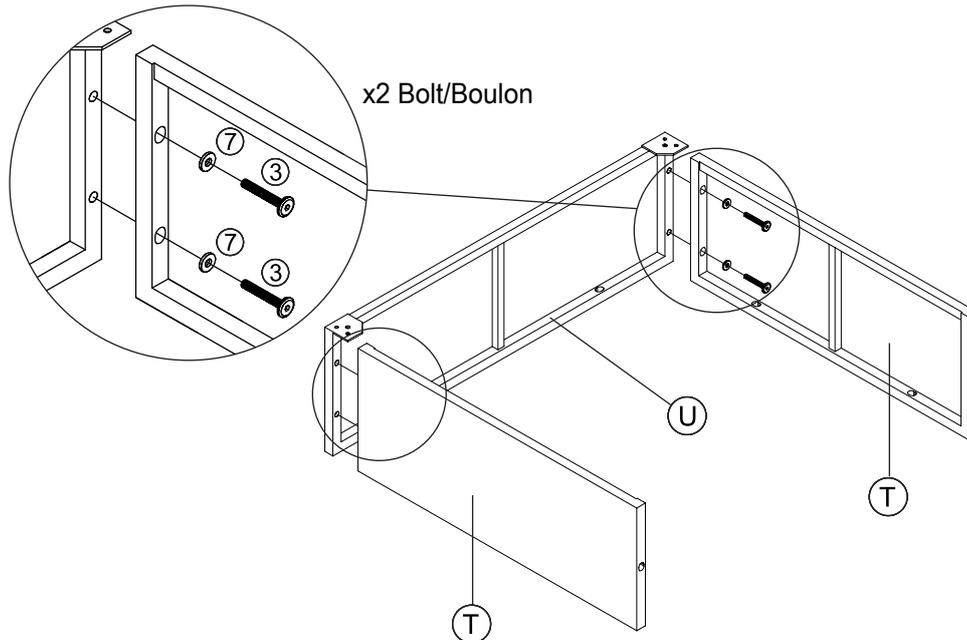
Connect the side stool (T) & leg stool (U), tighten bolt (3), flat washer (7) with allen key (14).
