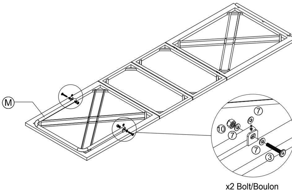
Connect the part from STEP 9 & support seat bench (M), tighten bolt (3), nut (10), flat washer (7) with allen key (14) & key (15).
