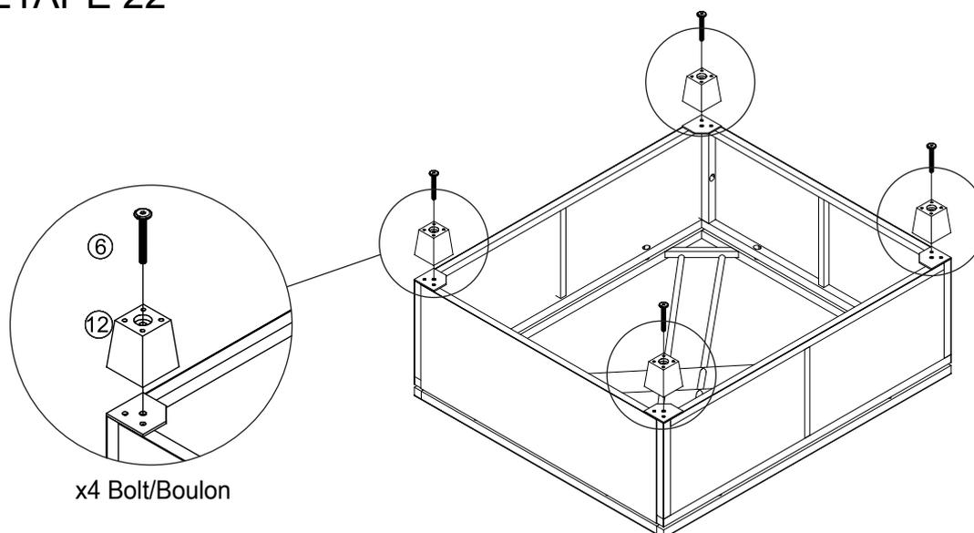
Connect the part from STEP 21 & plastic feet (12), tighten bolt (6) with allen key (14).
