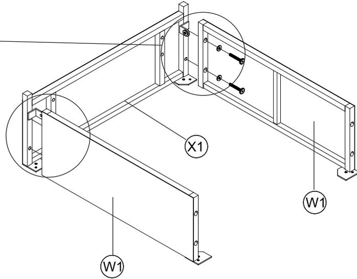
Connect the side table (W1) & Left leg table (X1), tighten bolt (3), flat washer (7) with allen key (14).
