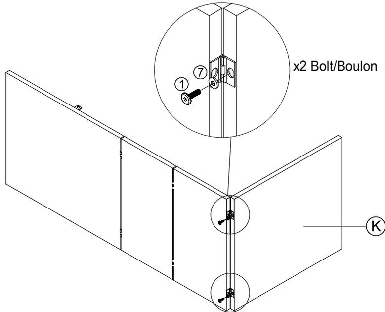
Connect the part from STEP 8 & front seat bench (K), tighten bolt (1), flat washer (7) with allen key (14).
