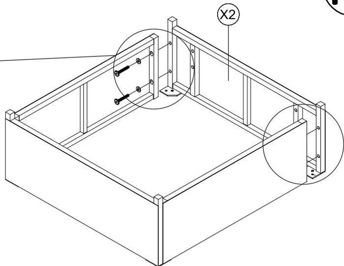
Connect the part from STEP 25 & Right leg table (X2), tighten bolt (3), flat washer (7) with allen key (14).
