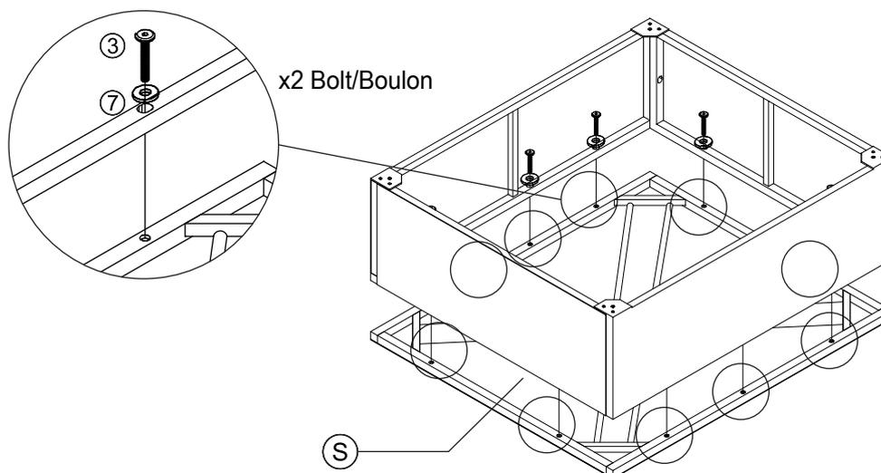
Connect the part from STEP 20 & top stool (S), tighten bolt (3), flat washer (7) with allen key (14).
