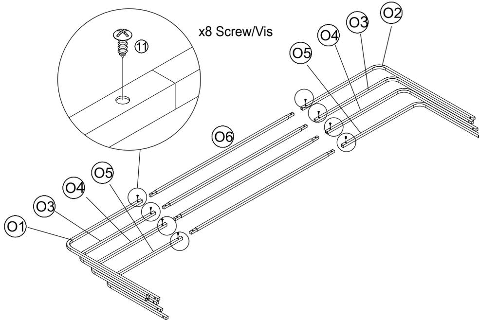
Connect the left support (O1), right support (O2), support (O3), (O4), (O5) & support (O6), screw (11).
