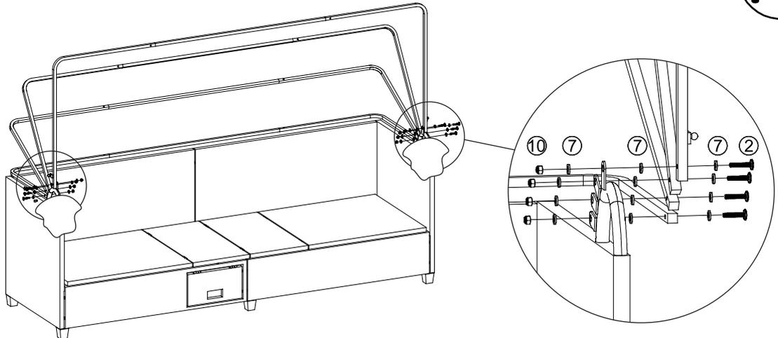
Connect the part from STEP 12 & with STEP 14, tighten bolt (2), nut (10), flat washer (7) with allen key (14), key (15).
