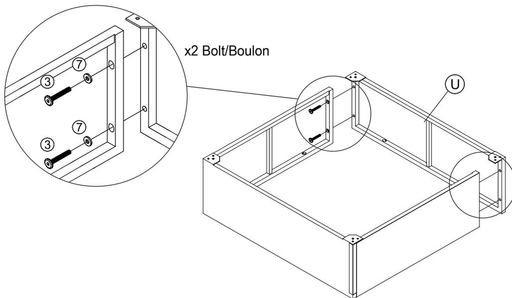
Connect the part from STEP 19 & leg stool (U), tighten bolt (3), flat washer (7) with allen key (14).
