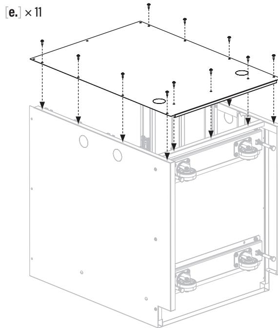
**STEP 07** Slide the countertop [8] into the cabinet panels. Use nine (9) large screws [e.] to secure.
