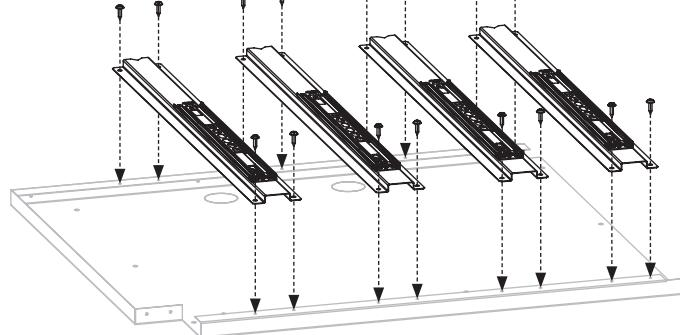
**STEP 04** Use sixteen (16) large screws [e.] to attach four (4) drawer slide mounts [11] to the left cabinet panel.
