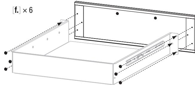
**STEP 11** Pull out the bottom two (2) drawer sliding tracks from the glide housing. Insert the drawer slides of one (1) large drawer into the cart tracks.
