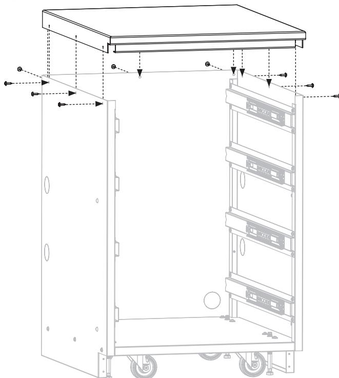
**STEP 08** Use four (4) large screws [e.] to attach the toe kick [5] to the left and right cabinet panels.
