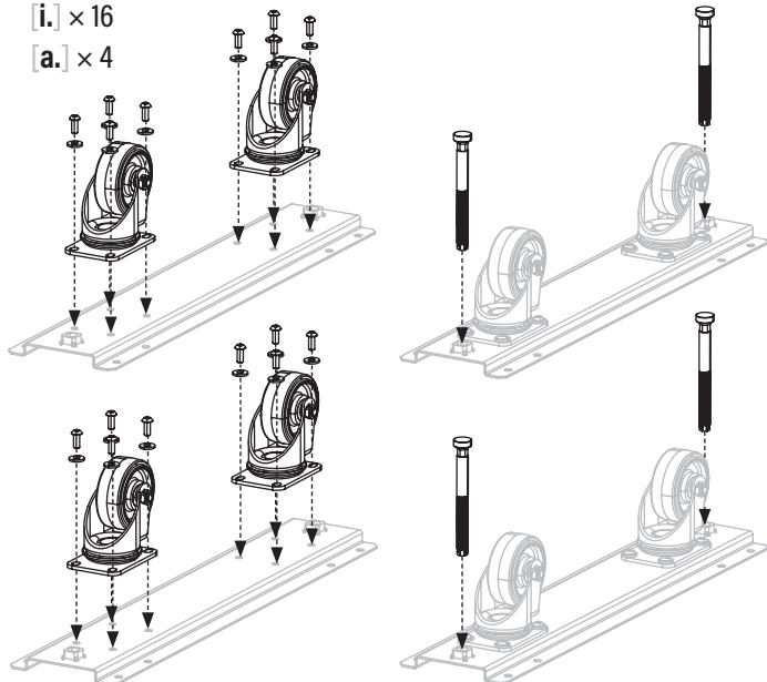
**STEP 02** Use eight (8) zinc bolts [i.], eight (8) zinc washers [g.], and eight (8) zinc lock nuts [h.] to attach the caster plates to the underside of the cart base [4].
