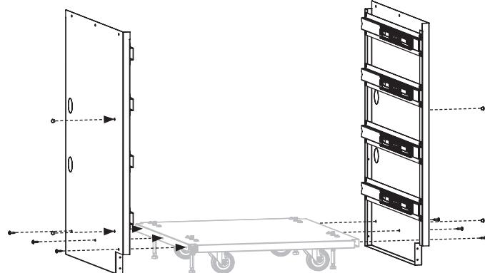
**STEP 06** Use eleven (11) large screws [e.] to attach the rear cabinet panel [3] to the left and right cabinet panels.
