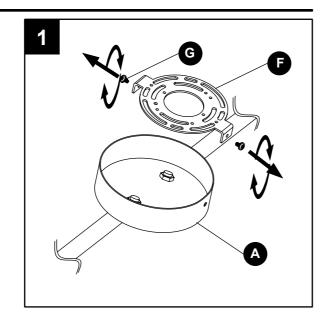
2. Fasten the mounting bracket (F) to the outlet box with outlet box screws (BB).
