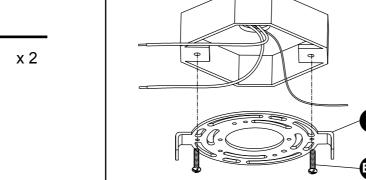
3. Strip 3/4 in. of insulation from wire ends. Connect white wire from fixture (A) to white wire from outlet box using wire nut (AA). Connect black wire from fixture (A) to black wire from outlet box using wire nut (AA). Connect bare/green ground wire from outlet box to bare ground wire from fixture (A) with wire nut (AA).
