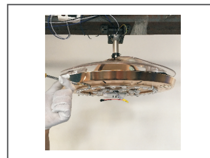
Step 4. Remove the screws on the side of the main engine chassis mounting attachment.
