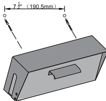
For brick or other masonry walls, insert the anchor into the wall. Install screws, ensuring to leave a gap of 1/4" between wall and screw head. Anchors are not needed for a wood wall.
