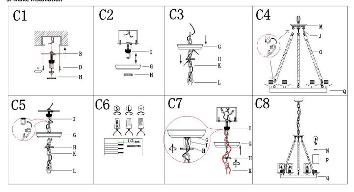
Step C1: .Attach single bar (B) to outlet box with mounting screws (D). The side of single bar marked "GND" must face out Step C2: Raise the canopy (G) through screw collar loop (I) and screw the collar loop (I) to a proper position by measuring .
