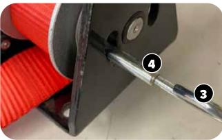
Screw in the provided tool 3 and pull the pin free from the winch. Once removed, you will be able to pull the strap away freely.
