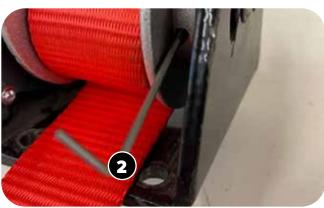
Remove the screw using an allen key 2 and set aside. Do not lose the screw, as you will need it to reinstall your new winch strap.
