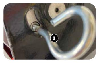
Use the tool that was provided in your plow kit 3 to begin removing the winch pin (you may be able to use needle nose pliers as well)
