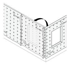
**STEP 4** Fasten the side flaps and secure the bottom flap to the foundation. For maximum air leakage reduction (when installing as an air barrier), seal wrap at the bottom of the wall with DuPont™ Weatherization Sealant, DuPont™ Tyvek® Tape or DuPont™ StraightFlash™.
