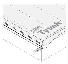
**STEP 3** As each wall section is raised, ensure that the bottom flaps overlap the sill plate and that the side flaps are on the exterior of the house.
