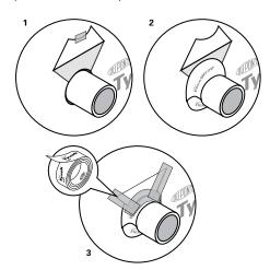
Products that have flanges should be integrated into the water-resistive barrier using DuPont™ Tyvek® Tape or DuPont™ Flashing Systems products.
