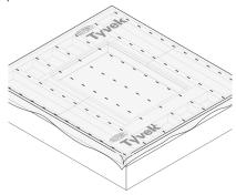
**STEP 2** When starting a wall section, fold the beginning side flap over the vertical side of the stud and secure. Trim off excess. Ensure that the bottom flap overhangs enough so that, when the wall is tilted upright, it overlaps the sill plate.
