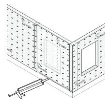
**STEP 5** All vertical seams shall be taped with DuPont™ Tyvek® Tape. For maximum air penetration resistance, when installing as an air barrier, all horizontal seams shall also be taped.
