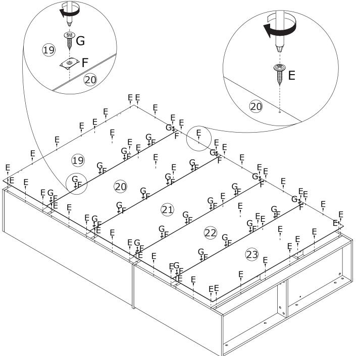
Fix back board 19, 20, 21, 22 and 23 to cabinet with screw(E) as shown. Use iron sheet(F) to fix each back boards with screw(G) as shown.
