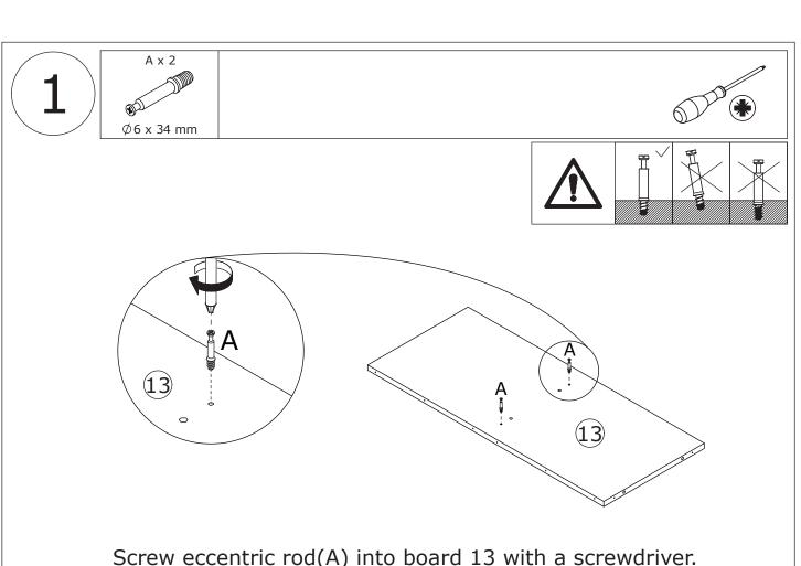
Screw eccentric rod(A) into board 13 with a screwdriver.
