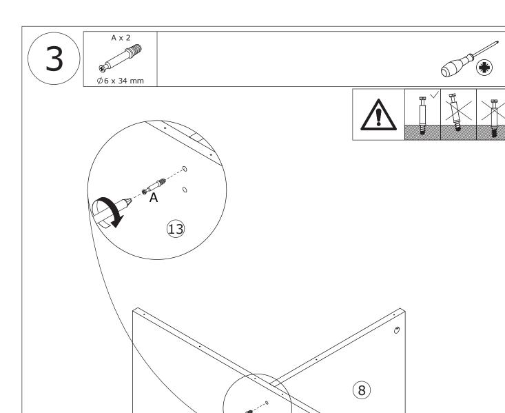
Screw eccentric rod(A) into board 13 with a screwdriver.
