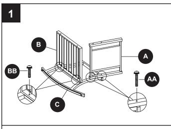
Hand tighten AA and BB. Do not tighten with wrench CC, until all bolts have been installed.
