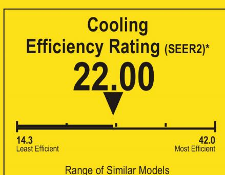
efficiency ratings depend on the coil your contractor installs with this unit. The heating efficiency rating varies slightly in different geographic regions. Ask your contractor for details.
