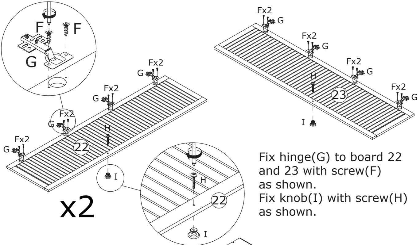
Fix hinge(G) to board 22 and 23 with screw(F) as shown.
