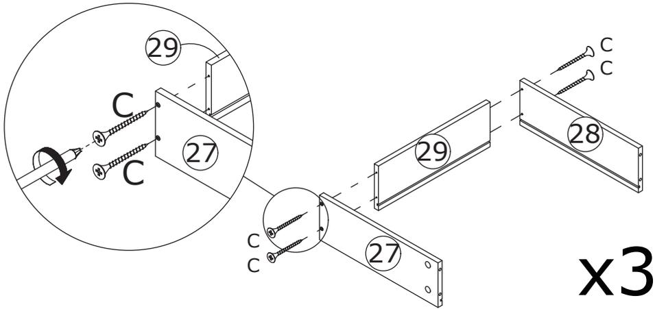
Fix board 27 and 28 to board 29 with screw(C) as shown.
