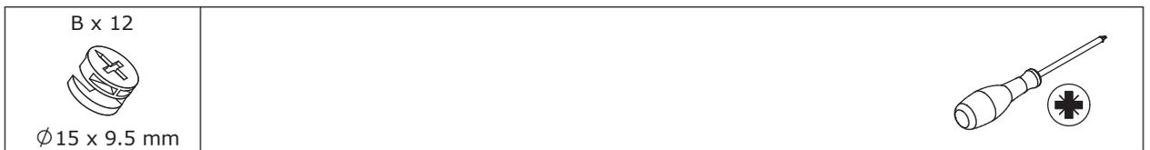
Attach board 13, 31 and 36 to board 27 and 28, add cam lock(B) and turn clockwise to tighten as shown.
