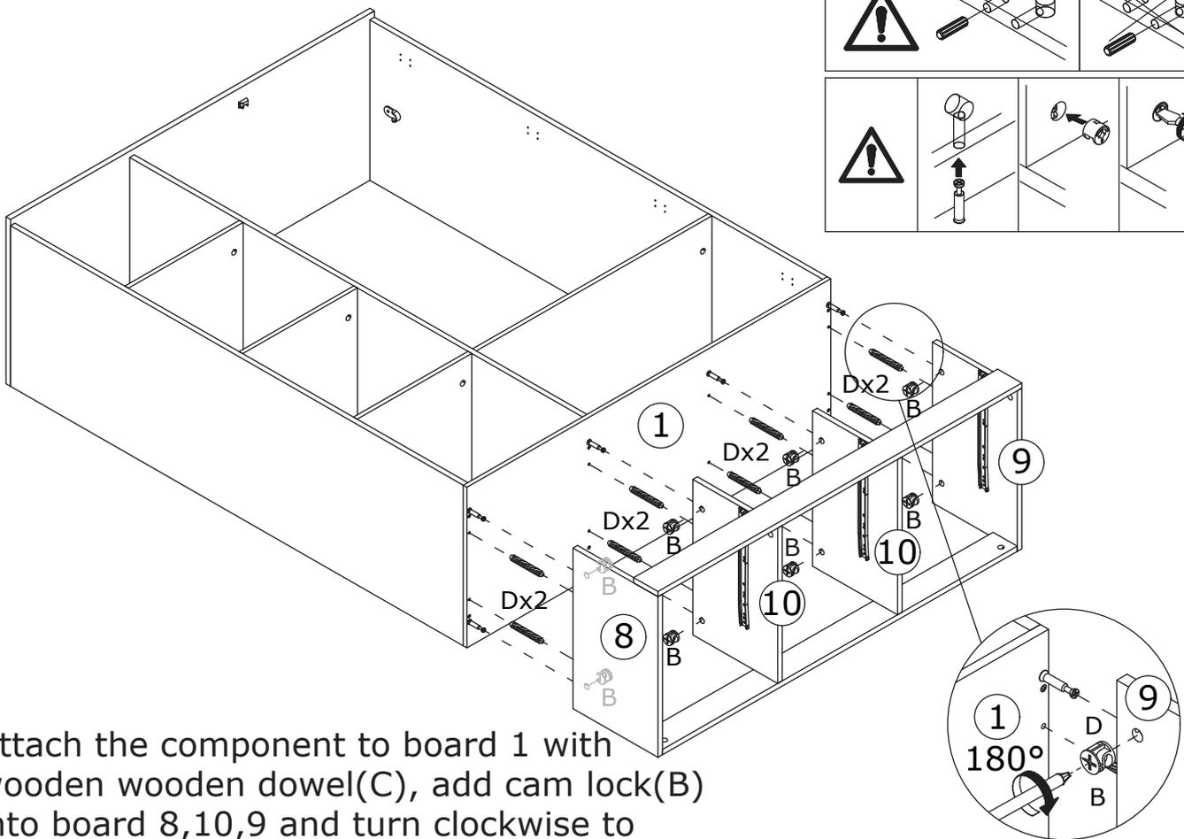
Attach the component to board 1 with wooden wooden dowel(C), add cam lock(B) into board 8,10,9 and turn clockwise to tighten as shown.
