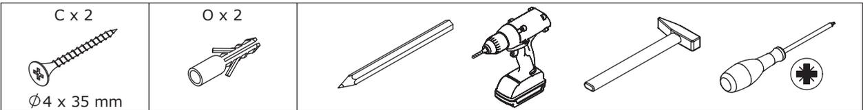
Once assembled lift furniture into place, do not drag. Use a drill to create a small hole lining up with the top of the safety strap (M). Fasten to wall using wall anchor (O), wall screw (C). Ensure the unit is balanced and steady before use. You're done, enjoy
