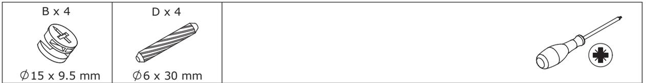
Attach board 12 to board 8, 10 and 9 using wooden dowel(D), add cam lock(B) into board 8,10,9 and turn clockwise to tighten as shown.
