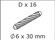
Insert wooden dowel(D) into board 5 and 6 as shown.
