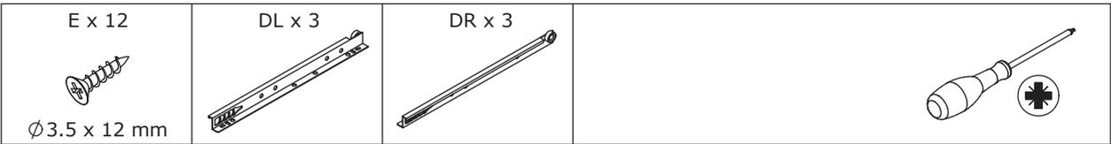
Fix runner(DL) and (DR) to board 27 and 28 with screw(E) as shown.
