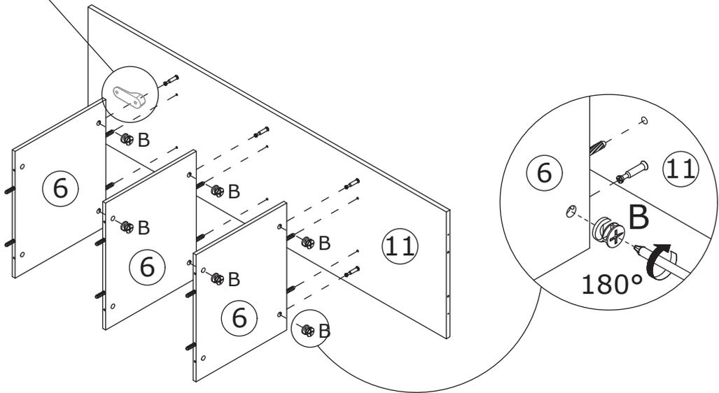
Attach board 6 to board 11, add cam lock(B) into board 6 and turn clockwise to tighten as shown.
