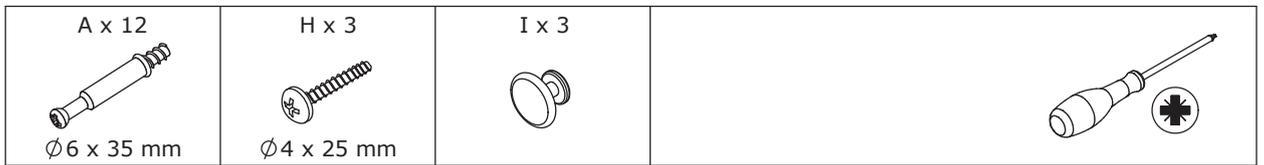
Screw eccentric rod(A) into board 13, 31 and 36 at first.
