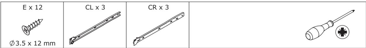
Fix rail(CL) and (CR) to board 8 and 9 respectively with screw(E) as shown. Fix rail(CL) to board 10 with screw(E) at first, flip to back, fix rail(CR) as shown.
