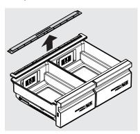
**Removing Auto Humidity** Control Membrane
