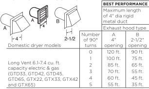
For every extra 90° elbow, reduce the allowable vent system length by 10 ft.
