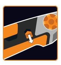
6. Push the lock down into the locked position.
