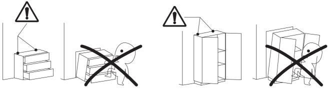
Once assembled lift furniture into place, do not drag. Use a drill to create a small hole lining up with the top of the safety strap (M3). Fasten to wall using wall anchor (L), washer (M2), wall screw(C). Ensure the unit is balaced and steady before use. You're done, enjoy
