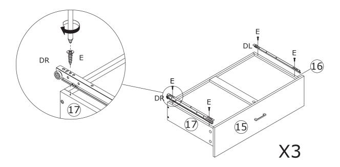
Fix track(DL) and (DR) to board 16 and 17 with screw(E) as shown.
