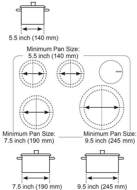
Use the cross that marks each cooking element to help determine the maximum pan size. After centering the cookware on the cooking element, the cookware should not extend more than  $\frac{1}{2}$ " beyond the edge of the cross on the cooking element. The pan must make full contact with the glass surface without the bottom of the pan touching the metal cooktop trim.
