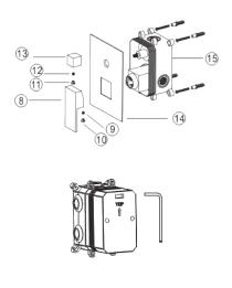
Please fix the ®Main body to the wall then remove the plastic protective cover and install ®Panel ® Water diverter, ® Screw,® Water diverter cup in the order. Finally you could install ® Handle, ® Screw, ® Handle cup.
