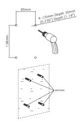
According to the size of installation to install the anchors to the wall. Please note that the levelmeter should be parallel, otherwise the panel cannot be installed Pay attention to the length and width of the screw position before marking
