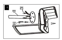
Step 4 Align the column (D) onto middle of the frame as pictured. Place the assembled seat onto the base Use allen key "H4" to lock the 4 screws "H2".
