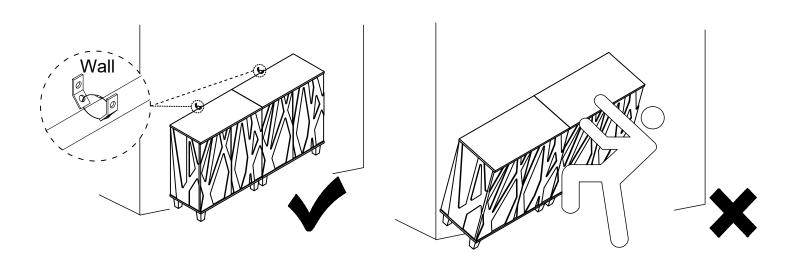
( Install tip-over restraint provided) Use of tip-over restraints may only reduce but not eliminate, the risk of tip-over.
