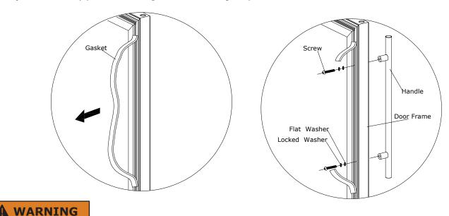
Improper gasket installation will result in condensation
