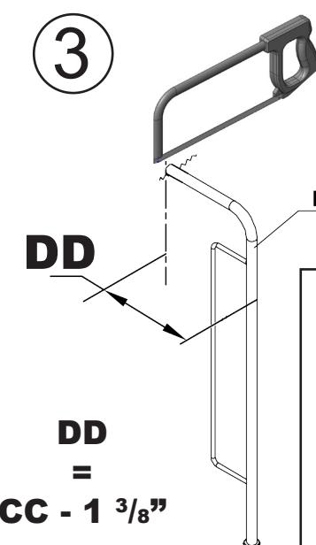
All banisters except the top, take the measurement of CC and reduce it by 1 3/8" (per DD) to cut handrail to the proper length. Drill holes in tread 1 1/8" from front and 1 1/8" edge of tread and install top banister.
