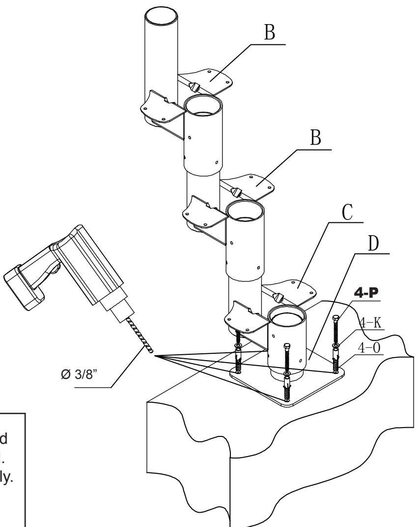
Install base into floor with screws and anchors depending on floor material. Anchor sleeves (4-O) for concrete only. Once completed, remove support.
