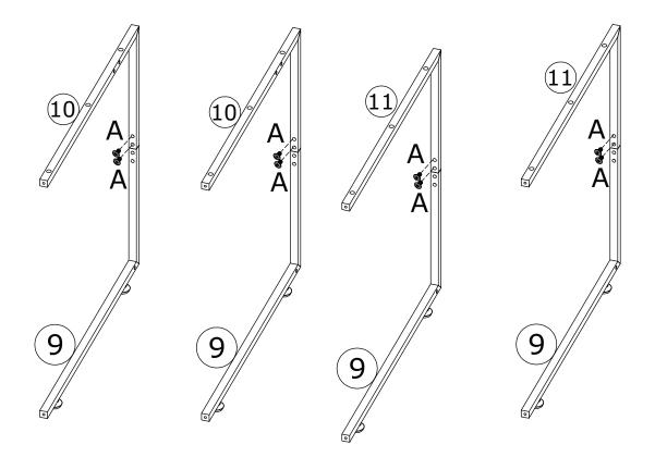
Fix each part together using screw(A) as shown.
