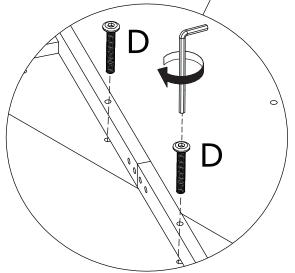
Fix the component to countertop using screw(D) as shown.
