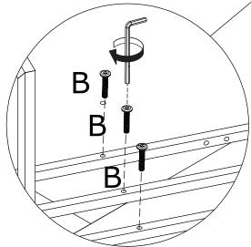
Fix part 10 and 11 to board 1 and 2 using screw(B) as shown.
