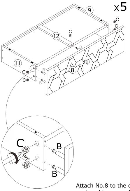
Attach No.8 to the component and turn cam lock(C) clockwise to tighten as shown.
