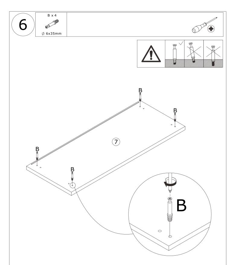
Insert quickfit screw(B) into No.7 plate with a screwdriver as shown.
