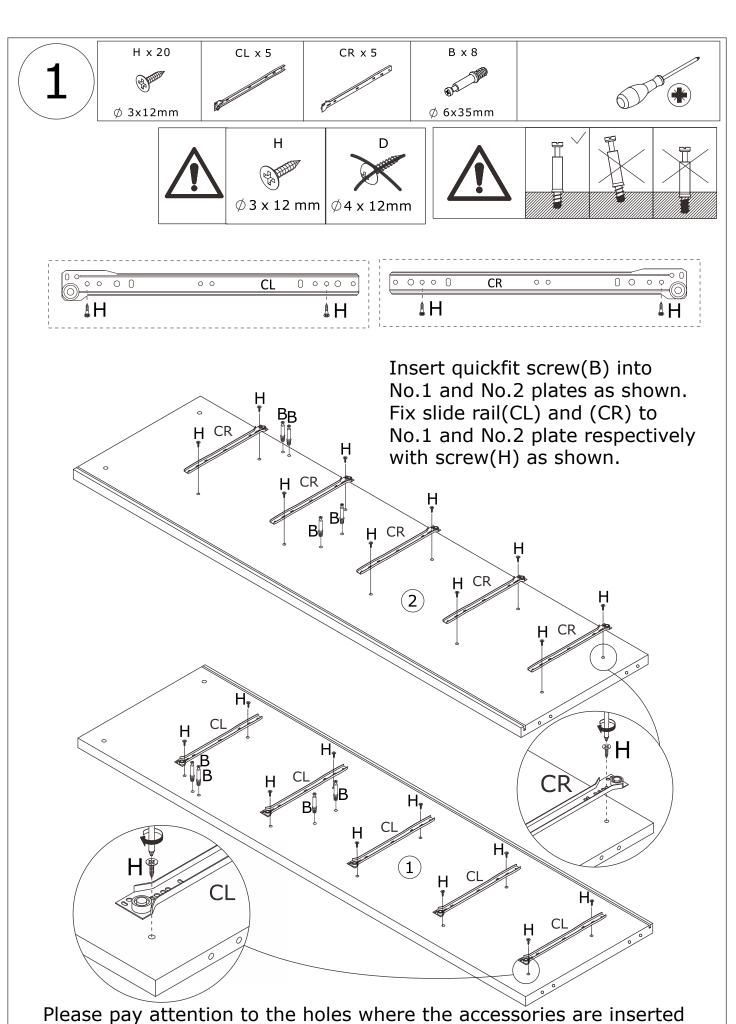
and don't use an electric screwdriver or use force to rotate, may cause crack.  $_{6/21}$
