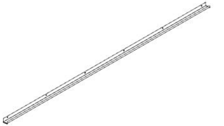
G06 GUTTER - A4M03481 (x2) 1 9/16"x1 15/16"x111 3/4" (40x50x2839)
