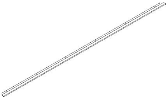
G01 GUTTER - A4M03478 (x1) 1 9/16"x1 15/16"x1117 5/16" (40x50x2838)
