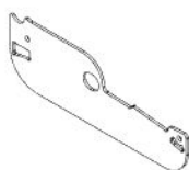
L03 LOUVER SIDE PLATE - A4M04138 (x66) 1/16"x2 3/16"x6 9/16" (2x55x167)
