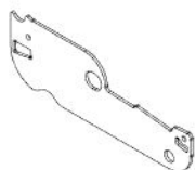
L02 LOUVER DRIVE SIDE PLATE - A4M04139 (x2) 1/16"x2 3/16"x6 9/16" (2x55x167)
