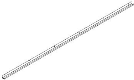
G02 GUTTER - A4M02583 (x1) 1 9/16"x1 15/16"x111" (40x50x2820)
