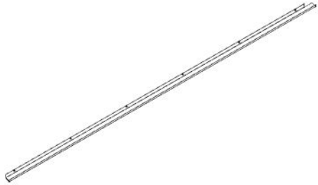
G01 GUTTER - A4M03478 (x1) 1 9/16"x1 15/16"x1117 5/16" (40x50x2838)
