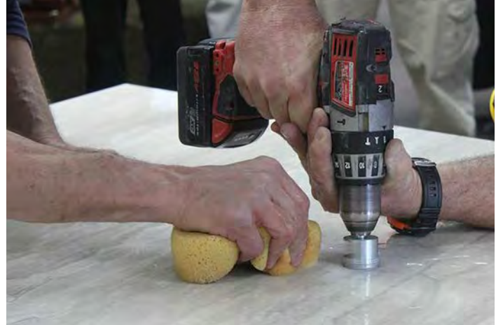
Image shows use of drill with electroplated diamond core bit.
