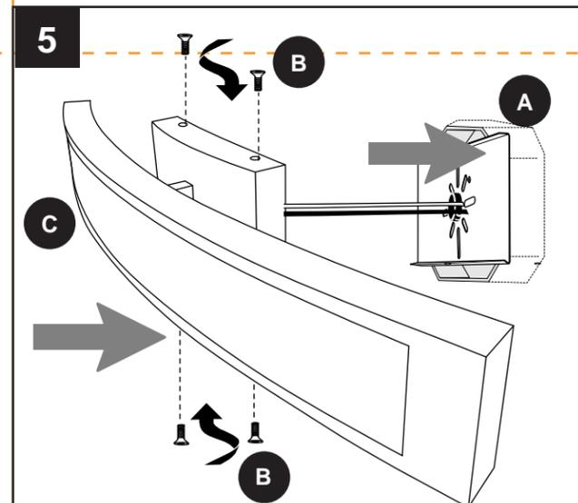
Before tightening B completely, use level (not included) to check C -- adjust if necessary.
