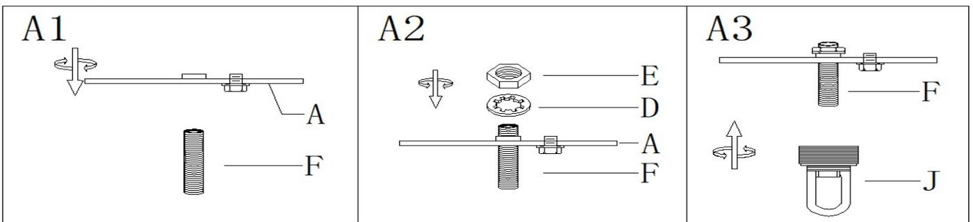
Step A1: Thread the single bar(A) onto the nipple (F), At this point need note that: the side of single bar marked "GND" must
