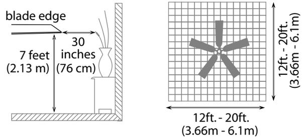
This fan can be mounted with a **downrod** on a regular (no-slope) or vaulted ceiling. The hanging length can be extended by purchasing a longer downrod (0.5in./1.27cm diameter). Other installation, such as **flushmount**, is *not* available for this fan.
