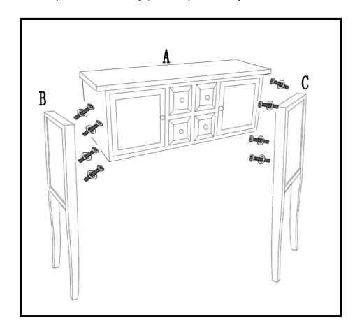
**Step 1**Attach the 2 Legs (B) (C) to the Top (A), open the doors
