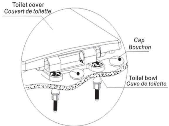
2. Insert the nut into the two holes perfectly and screw it with screwdriver, then put the cap on it.
