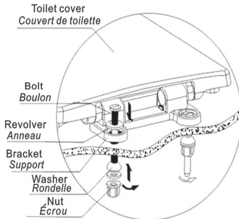
1. Insert revolver, washer and bolt into the installing hole.
