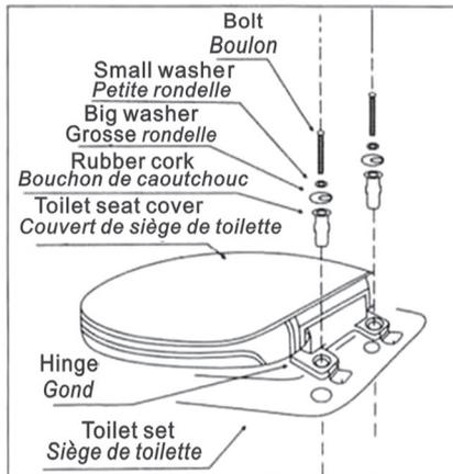
1. Place the toilet seat cover on bowl, insert the bolt, washer and rubber cord in hinge install hole-order;
