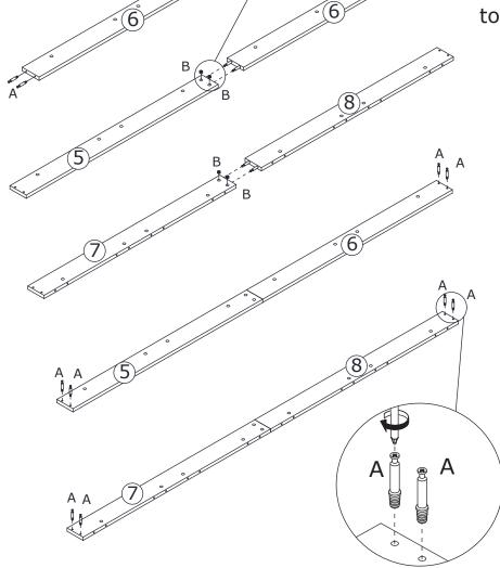
Screw eccentric rod(A) into board 5, 6, 7 and 8 as shown.
