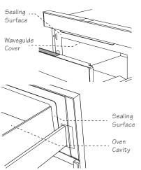
2 Remove the feature sticker, if there is one. Check the drawer for any damage, such as misaligned or bent
