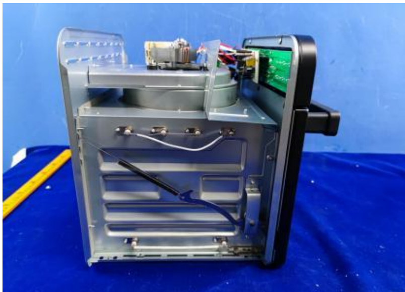
Photo 10 - internal view for control panel
