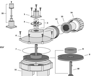
The knob on top of the cam has an arrow which points to the active zone. When the pump is turned off, index the cam to the desired zone by pushing down on the Zone Indicator. When the pump is turned back on the system will automatically start on that zone. This optional item for the Hydro-Indexing Valve is great to use when working on sprinkler heads. All valves with a threaded inlet as well as the all-metal valves are Zone Indicator ready.
