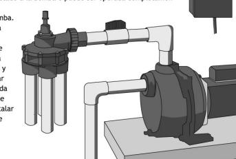
On a city water installation, no less than a one inch solenoid and one inch pipe leading into the valve should be used. A gate valve can be used for manual operation. For fully automatic operation, an electric solenoid and an electric timer must be installed. On a 1 1/2" or larger meter, the manufacturer recomends that an all metal valve should be used.
