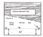
**Note:** This dimension should be 4" when installing 3 ¼" wide flooring. When a room is greater than 20 ft. in width, the direction of the installation should start near the center of the room and work out towards the walls placing a loose spline where the two grooves come together.
