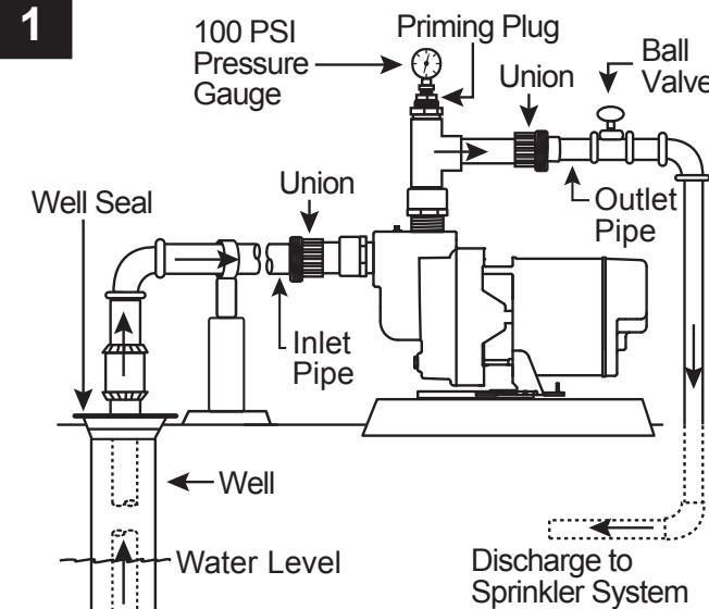
2. Glue female 2 in. union (not included) to the end of inlet pipe leading from the water source.
