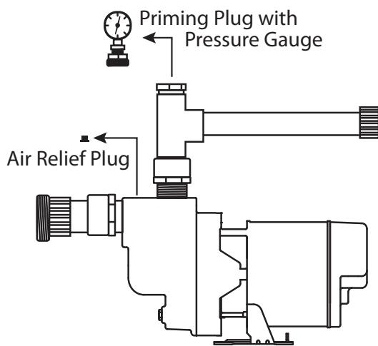
3. Slowly fill pump cavity until water comes out of air relief hole on top of the pump.
