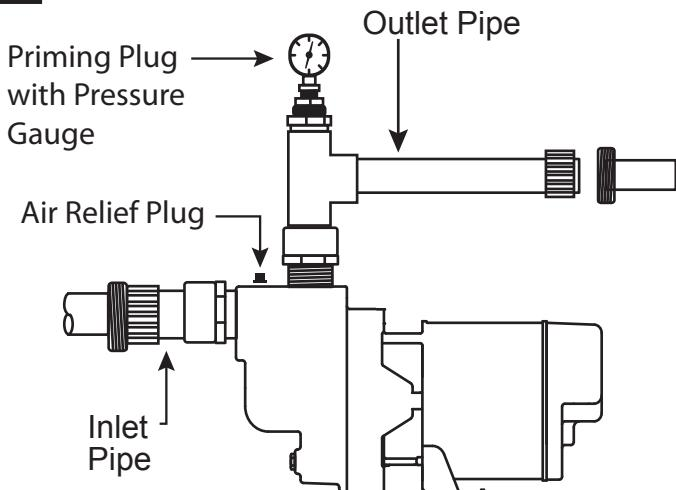
2. Remove the air relief plug on top of pump and the 1-1/4 in. priming plug with pressure gauge or plug. Refer to Pump Preparation Step 5.
