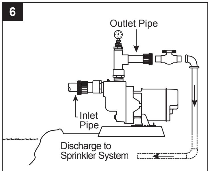
7. Connect union to ensure proper fit. Do not tighten until after priming.
