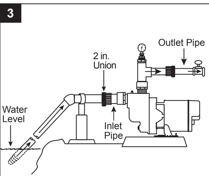
4. Glue a 6 in. piece of 1-1/2 in. pipe (not included) to the female portion of the 1-1/2 in. union.
