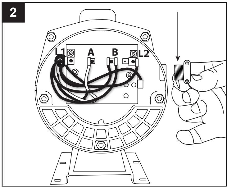
3. Insert wire through electric wire strain relief and tighten screws.
