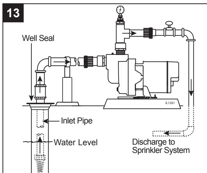
14. Glue a 90° elbow (not included) when the inlet pipe is in line with the inlet port of the pump.
