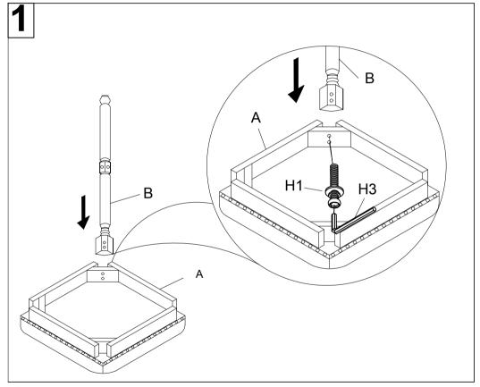
Step 1: Attach 4\* legs (B) and cushion (A) ,use Allen key (H3) to lock with 8\*Allen bolt (H2).
