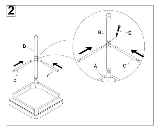
Step 2: Attach 4\* stretcher (C), use screw driver to lock with 8\*screw (H2). Straighten up the assembled product, assembly is completed.
